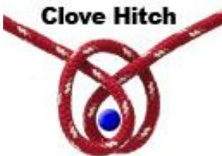
The Clove Hitch can be done in two ways. It can be done with two loops on a bite of rope or it can be done at the end of the rope. The Clove Hitch has two glaring faults: in some applications it may bind and be hard to undo; and, in others, it may slip under load. It can be used for adjusting the height of tent ropes or tarp ropes.
